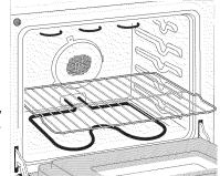
Installing Oven Rack Supports in Upper Oven
