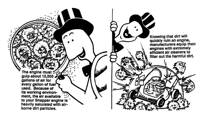
As the dirt particles are stopped, they build up and begin to clog the outside of the filter. This reduces the amount of air available to the engine and causes an over-rich fuel mixture which results in the following adverse effects:
