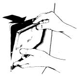
Tip the window and frame out from the top slightly.
