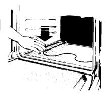
For proper baking, lower the bake element so all feet rest solidly on the foil.
