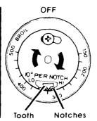
4. To raise the temperature, move black ring so tooth is closer to HI. Each notch equals about 10 F (5 C).
