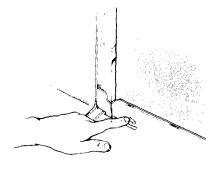
When the hinges snap into place, open the door and move the broil stop clips. Close the door.
