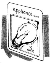
Replace the bulb with a 40-watt appliance bulb available from most grocery, variety and hardware stores. Turn electrical power back on at the main power supply.
