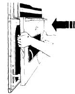
Carefully push the hinges straight in while lifting slightly on the door.
