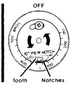
To lower the temperature, move black ring so tooth is closer to LO. Each notch equals about 10°F (5°C).
