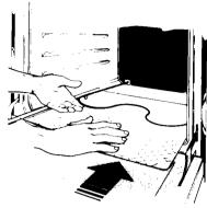
Slide the foil under the bake element.
