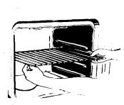
Lift rack at front and pull out
