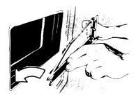
Fit the bottom tabs of the frame into the bottom of the window opening.
