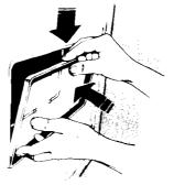
Push the top of the frame into the opening while pushing down.
