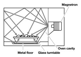
**Microwaves** pass through most glass, paper, and plastics without heating them so food absorbs the energy. Microwaves bounce off metal containers so food does not absorb the energy.
