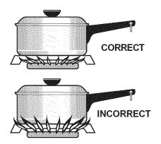
Never extend the flame beyond the outer edge of the utensil. A higher flame simply wastes heat and energy, and increases your risk of being burned by the flame. **For most cooking**, start on the highest control setting and then turn to a lower one to complete the process. Use the recommendations below as a guide for determining proper flame size for various types of cooking. The size and type of utensil used and the amount of food being cooked will influence the setting needed for cooking.
