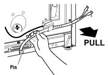
**STEP 2.** Pull firmly to remove the end of the shipping strap that remains pinned to the back of the washer. This will release the rear self-leveling legs.
