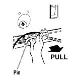
**STEP 3.** Cut the shipping strap about 16 in (40 cm) from plug end. Look for the words "CUT HERE." Discard end with the cotter pins. **Slide remainder of shipping strap from the electrical plug.** You will use this to secure the drain hose.
