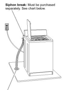
Floor drain system: Requires a siphon break, see chart below. A minimum carry-away capacity of 17 gal (64 L) per minute is required.
