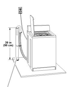
Standpipe drain system: Needs a 2-in (5 cm) minimum diameter standpipe with minimum carry-away capacity of 17 gal (64 L) per minute. Top of standpipe must be at least 39 in (99 cm) above floor and no higher than 96 in (2.4 m) from bottom of washer.
