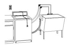
**STEP 2.** Locate the remaining piece of shipping strap (not the end with the cotter pins) from STEP 3 of "REMOVE SHIPPING STRAP." Use it to wrap the drain hose together with the laundry tub or standpipe. Push fastener into the nearest hole in the shipping strap.
