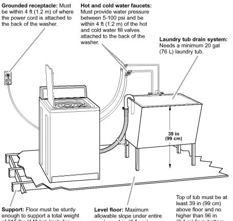
of 315 lbs (143 kg) (includes washer, water, and load weight). washer - 1 in (2.5 cm).
