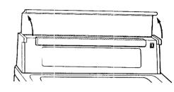
STEP 3. Pull off and remove the plastic light cover.
