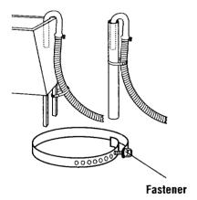
If the water faucets and drain standpipe are recessed, put hooked end of drain hose in standpipe. Tightly wrap the shipping strap around the drain hose and water inlet hoses (not the handles or stems). Push fastener into the nearest hole in the shipping strap.
