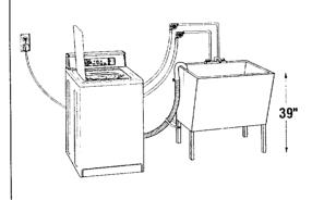
Standpipe Drain System (p. 12)
