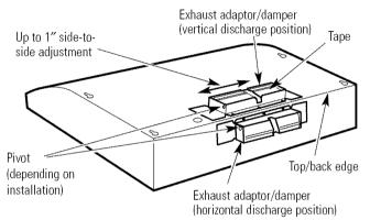
**NOTE:** The exhaust adaptor/damper can be installed up to 1 inch on either side of the hood center to accommodate off-center ductwork. In extreme offcenter installations, one end of the duct connector may need to be trimmed to clear the electrical cable clamp.
