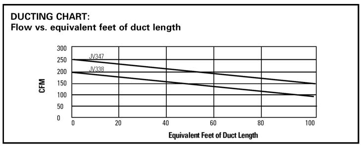
**MAXIMUM DUCT LENGTH:** For satisfactory air movement, the total duct length of a 3<sup>1</sup>/<sub>4</sub>" x 10" rectangular, 6" or 7" diameter round duct **should not exceed 65 equivalent feet.**
