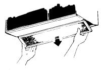
Push in the two filter fasteners at the back edge of the filter.
