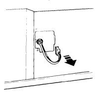
1. Remove filter, light lens and fluorescent cooktop lamp as described above. Pull down on the white connector plug to disconnect.
