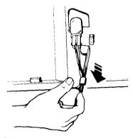
2. Remove the oven light cover screw, slide the light cover off and pull the oven light assembly out of the oven cavity.
