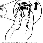
**3.** To remove the starter, push in and twist it to the left. To replace the starter, push in and twist it to the right.
