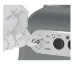
\* To start the Chef's Blender at the Medium (Med) or High speed settings, move the On/Off/Pulse Switch to the "On" position while pressing the desired Speed Selection Button.
