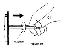
Slide washer along straps until inner rim of washer seats completely inside of drilled hole. (See figure 11.)
