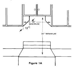
\*If this microwave/hood is installed in cabinetwork that extends beyond 13" (see Figure 1A) or along a side wall that extends more than 13", an extra one inch will be required for proper door opening clearance. See Figure 1B.
