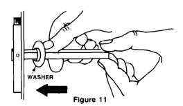
Snap off plastic straps flush with washer. (See figure 12.)
