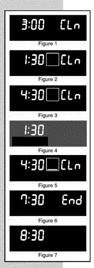
To set the control for the Self-Cleaning Cycle to start at a delayed time and shut off automatically: (example 3 hour self-clean cycle to start at 4:30).
