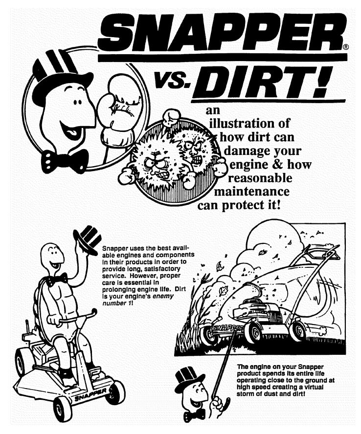
The engine must guip about 12,000 gallons of air for every gallon of fuel used. Because of its working environment, the air available to your Snapper engine is heavily saturated with airborne dirt particles.
