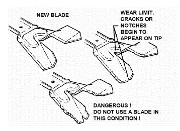
2. Replace the blade if it is badly chipped, bent, noticeably out of balance or has cracks or notch in either tip. See Figure 4.1 & 4.2. Replace with new blade.
