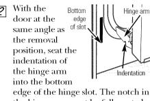
the hinge arm must be fully seated into the bottom of the slot.
