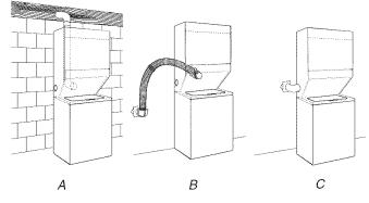
A. Standard rear offset exhaust installation
