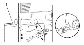
5. Place clamp over the area marked "CLAMP." Release clamp.
