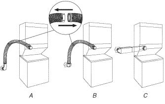
A. Loop system with standard elbows B. Loop system with one offset and one standard elbow
