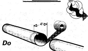
Use 4 inch diameter rigid metal duct. Tape all joints. Never use lint-trapping screws.
