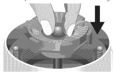
2. Place the grind-adjustment ring onto the motor housing. Press and turn the grind-adjustment ring clockwise several rotations until the gear offers complete resistance, then rotate it counterclockwise until the selection arrow aligns with the initial "M" for the Medium grind selection.
