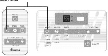
Once the function mode is decided you will have to set the fan speed.(See fig. #4) Every time you press the SPEED button, fan speed will change between LOW, HIGH,MED.
