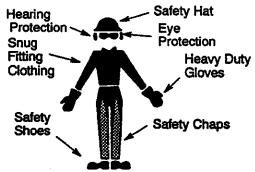
Wear protective gear. Always use steel-toed safety footwear with nonslip soles; snug-fitting clothing; heavyduty, non-slip gloves; eye protection such as non-fogging, vented goggles or face screen; an approved safety hard hat; and sound barriers (ear plugs or mufflers) to protect your hearing. Regular users should have hearing checked regularly as chain saw noise can damage hearing. Secure hair above shoulder length.
