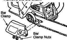
Turn adjusting screw on bar to move the tensioning rack as far as it will go toward the front of the bar.
