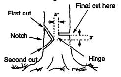
After removing the wood, make the felling cut on the opposite side of the notch. This is done by making a cut about two inches higher than the center of the notch. This will leave enough uncut wood between the felling cut and the notch to form a hinge. This hinge will help prevent the tree from falling in the wrong direction.
