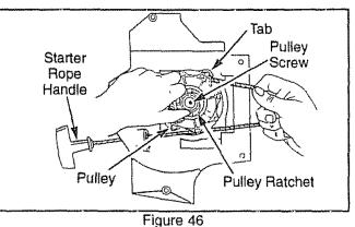
Remove the rope retainer screw and remove any remaining rope.
