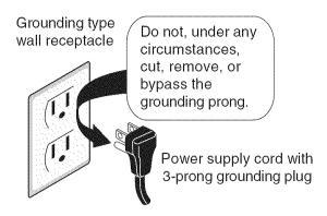
A WARNING Avoid fire hazard or electrical shock. DO NOT use an adapter plug, an extension cord, or remove grounding prong from electrical power cord. Failure to follow this warning can cause serious injury, fire or death.
