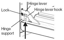
Lock engaged for door removal Figure 1
