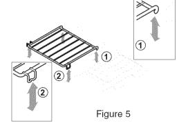
items. The right half rack portion may still be used for other food items like a casserole dish (See Figure 3). To remove the insert, squeeze on the left front insert side (See Figure 4) of the rack and tilt out clockwise. To reinstall insert rear hooks at back of insert (See Figure 5) and lay insert down. Make sure both insert front hooks snap into rack (See Figure 5).
