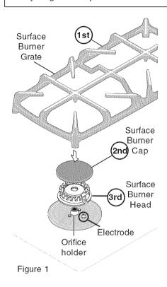
**To Remove and Replace the Surface Burner Caps and Burner Heads -** Remove in the following order: (1st) surface Burner Grates, (2nd) Burner Caps and (3rd) Burner Heads. Replace in the following order: Burner Heads, Burner Caps and Burner Grates.
