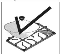
Woks with flat bottoms suitable for use on your cooktop are available in most cookshop or hardware stores. Round-bottomed woks (with a support ring that does not extend beyond the burner circumference) may also be used. The metal ring was designed to support the wok safely when it is filled with large amounts of liquids (soup making) or fat (frying).
