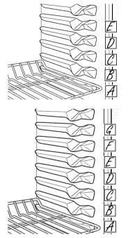
30" Trivection™ oven has 5 rack positions A–E (as shown). 30" lower oven of double oven has 7 rack positions A–G (as shown).
