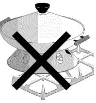
Improper use of round-bottom wok on Surface Burner Grate Figure 3
