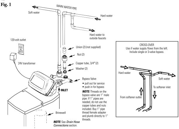
Optional 3-Valve Bypass Installation Illustration Adapters for this installation are not supplied with the softener. To order these adapters, call GE Parts 800-626-2000. Ask for part number WS60X10006.
