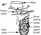
If you don't get a reading in the display, with faucet open, pull the sensor from the valve outlet port. Pass a small magnet back and forth in front of the sensor. You should get a reading in the display. If you get a reading, shut off water supply, unhook the in and out plumbing and check the turbine for binding.
