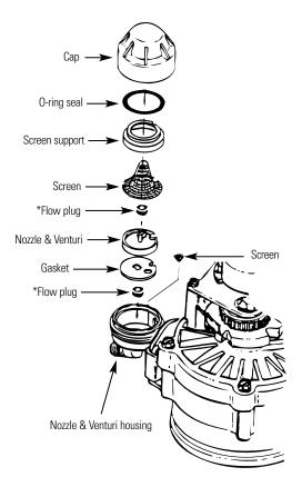
IMPORTANT: Be sure small holes in the gasket are centered directly over the small holes in the nozzle and venturi housing.
