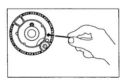
ACAUTION Use caution when replacing the burner cap so the electrode is not damaged. This may cause a delayed ignition or prevent the burner from igniting.
