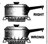
For most cooking, start on the highest control setting and then turn to a lower one to complete the process. Use the chart below as a guide for determining proper flame size for various types of cooking. The size and type of utensil used and the amount of food being cooked will influence the setting needed for cooking.
