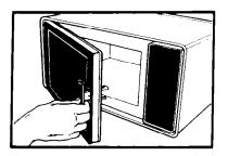
**1.** Open the oven door by lifting the door handle.
