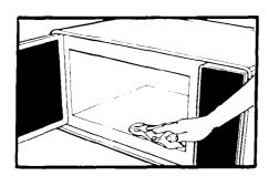
**1.** Empty the microwave oven and clean inside it with a soft, damp cloth. Check for damage such as misaligned door, damage around the door or dents inside the oven or on the exterior. If there is any damage, **do not** operate the unit until it has been checked by an authorized Whirlpool service technician and any repair made.
