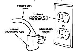
polarized 3-prong grounding plug. It must be plugged into a correctly polarized mating 3-prong grounding type wall receptacle, properly installed and grounded in accordance with the National Electrical Code and local codes and ordinances. If a mating wall receptacle is not available or if you are not sure if the
