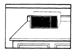
2. Put the oven on a cart, counter, table or shelf that is strong enough to hold the oven and the food and utensils you put in it. (The control side of the unit is the heavy side. Use care when handling.) The weight of the oven is approximately 39 lbs. (17.7 kg.).
