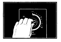
Set the cooking time by turning the Timer Knob clockwise. To reduce the cooking time, turn the Timer Knob counterclockwise.
