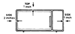
4. Do not install the microwave oven so that both sides and the top are flush with walls, shelves or cabinets. Leave clearance of at least 2 in. (5.08 cm) on the left side and 1 in. (2.54 cm) on the top and right side for proper operation.
