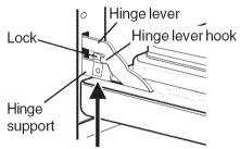
Lock engaged for door removal Figure 1
