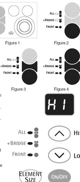
**Note:** If you bridge all three elements, any previous power level setting for the LEFT REAR element will be changed to the power level setting for the Bridge.
