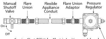
Service Shut-Off Valve Electric Ignition models only (Shown in ON Position).
