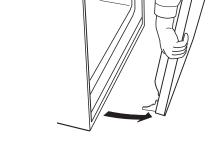
**2** ■ Completely open oven door. In both back corners of the door you will see door latches in the locked position. Rotate both latches forward to the unlocked position.
