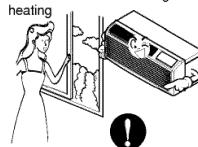
Do not insert hands or other objects through the air inlet or outlet during operation.
