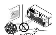
Do not block the inlet or outlet of air flow.
