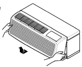
This Room Air Conditioner (PTAC) discharges air from the top of the unit through reversible, 2position discharge grille louvers. The unit is shipped from the factory with the discharge grille louvers at an angle of 40° off vertical. In an alternate position the louvers will be at an angle of 15° off vertical.
