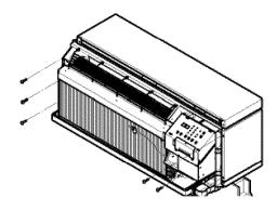
4. Reinstall the front grille by hooking the top over the unit top, then pushing it in at the bottom.
