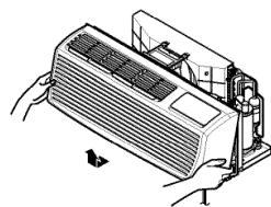
3. Slide the unit into the wall sleeve and secure with 6 screws through the unit flange holes.
