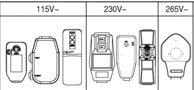
Power cord may include a current interrupter device. A test and reset button is provided on the plug case. The device should be tested on a periodic basis by first pressing the TEST button and then the RESET button. If the TEST button does not trip or if the RESET button will not stay engaged, discontinue use of the air conditioner and contact a qualified service technician.
