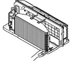
2. Remove the front gille by pulling it out at the bottom to release it, then lift it up along the unit top front.
