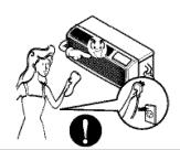
Take the power plug out if necessary, holding the end of the plug and do not touch it with wet hands.
