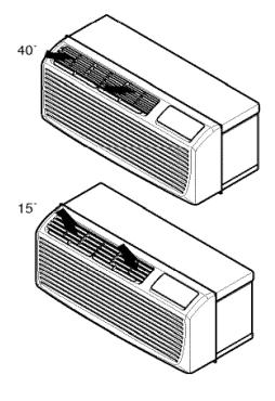
To adjust the air direction, remove the front grille. Remove the 4 screws that fasten the discharge grille to the front grille.
