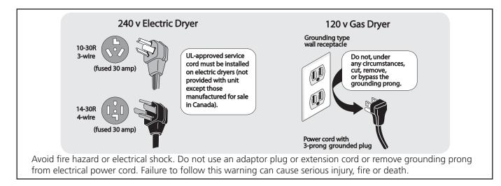
**WARNING** To reduce the risk of fire, electrical shock, or injury to persons when using this dryer, comply with the basic warnings listed below. Failure to comply with these warnings could result in serious personal injuries. You can be killed or seriously injured if you don't follow these Important Safety Instructions:
