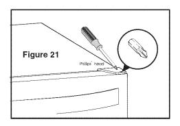
4 If door edge opposite the hinges needs to move up, move plate toward outside of door. If door edge needs to move down, move plate toward inside of door (see Figure 22). Repeat until top edge of door is parallel with top of cabinet and tighten screws securely.
