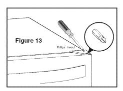
Remove plastic screw plugs (3 top and 3 bottom) from new hinge location (see Figure 14), and remove hinge pin hole plug in top of door (see Figure 15). Do not discard.
