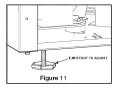
3 Check the levelness after each adjustment and repeat the previous steps until the unit is level.
