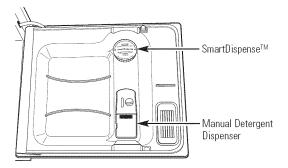
The cover of the main wash section will open during the wash cycle. If you are using SmartDispense™, leave the cover of the main wash section dispenser open before starting the cycle.
