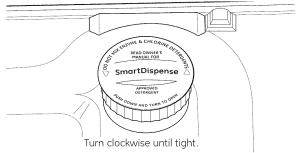
When full, replace the cap and turn clockwise until tight to ensure that no water enters the SmartDispense™ dispenser. If residue is left on the door, it will be washed off in the next cucle.
