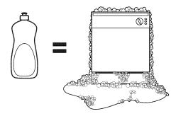
**NOTE:** Using a detergent that is not specifically designed for dishwashers will cause the dishwasher to fill with suds. During operation, these suds will spill out of the dishwasher vents, covering the kitchen floor and making the floor wet.
