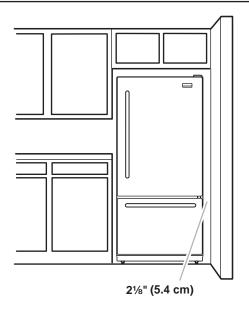
Your refrigerator does not require clearance on the top, back or sides. When installing your refrigerator next to a fixed wall, leave 2-1/8 in. (5.4 cm) minimum on each side (depending on your model) to allow for the door to swing open. If your refrigerator has an ice maker, allow extra space at the back for the water line connections.
