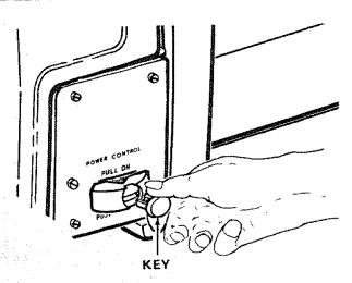
2. To turn Lathe ON . . . INSERT finger under switch lever and pull END of switch out.
