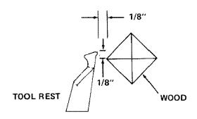
Look at the speed chart. Notice that a 2" square turning up to 18" long should run at 875 R.P.M. for "roughing". Move the V-belt on the pulleys to the slowest speed.
