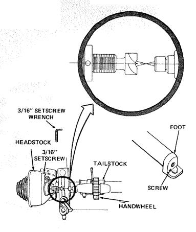
12. TAILSTOCK ... supports the workpiece for spindle turning.
