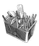
Be sure that thin, finely pointed items do not extend through the basket. This could block the lower wash arm.
