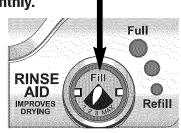
the cycle is adjustable by moving the lever inside the reservoir area. For most water conditions use the manufacturer recommended setting of "2". Adjust it up to the "MAX" setting for hard water. Set the lever anywhere between these amounts as needed to get the best results. Replace the cap and turn it clockwise to close.
