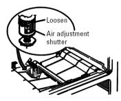
The shutter for the bottom (oven) burner is near the back wall behind the storage drawer or kick panel. Remove the drawer or panel. See the *Care and cleaning of the range* section.
