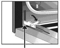
Lock engaged for door removal Figure 2
