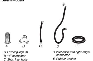
Remove parts package from dryer drum. Check that all parts are included.
