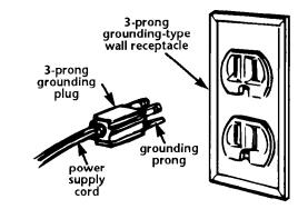
Local codes may permit the use of a U.L.listed, flexible, three-conductor, 16gauge, power supply cord terminated with a three-prong, grounding-type plug.
