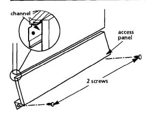
• Remove the 2 screws below the access panel. Pull bottom of panel out and lift up and away from dishwasher. Set access panel aside on a protective covering.
