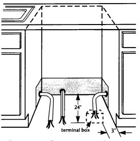
**3** • After dishwasher is installed in opening, remove terminal box cover.
