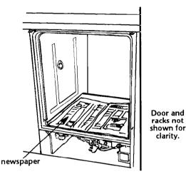
• Open dishwasher door and remove bottom rack. Remove all shipping materials, including foam shipping pieces from upper corners of door. Do Not remove the white plastic plug buttons from the side of the door or the plastic bumpers from the front corners of the lower rack. Place a newspaper or large sheet of paper over bottom of dishwasher to protect pump area when securing dishwasher to countertop.
