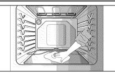
The bake element is designed to be tilted up using your hand from the front of bake element. This will allow easier access to the oven bottom for cleaning. Be careful not to raise the element more than 4 or 5 inches from the resting position.
