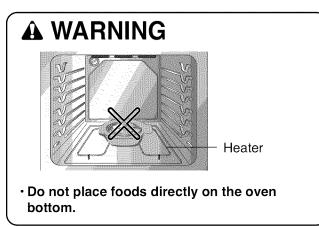
Doing so will cause permanent damage to the oven bottom finish.
