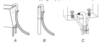
If the water faucets and the drain standpipe are recessed, put the hooked end of the drain hose in the standpipe. Tightly wrap the shipping strap around the water inlet hoses and the drain hose (C above). Push fastener into the nearest hole in the shipping strap (see illustration above).
