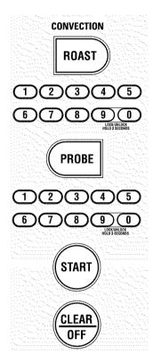
To change the oven temperature during the Convection Roast cycle, press the **CONVECTION ROAST** pad and then press the number pads to set the new desired temperature.
