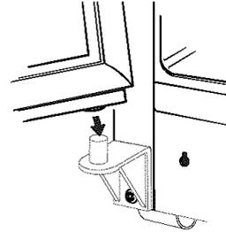
Straighten the door and line it up with the center hinge bracket.
