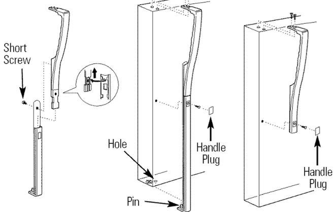
**After removing the handle:** Move the small plug buttons from the top right side of the door top and insert them into the holes on the opposite side.
