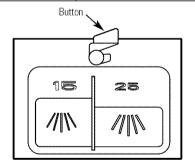
To open the wash cover, press the button and the cover will flip back.
