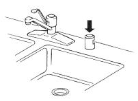
The drain air gap is usually located on top of the sink or countertop near the dishwasher. To order a drain air gap call your local dealer, or in the U.S.A., call the Customer Interaction Center and ask for Part Number 300096.
