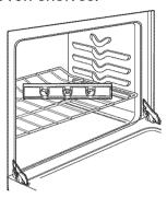
B Turn the legs counterclockwise to raise the range and counterclockwise to lower the range. Adjust the leveling legs until the range is level.
