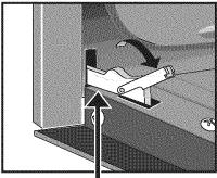
Lock engaged for door removal
