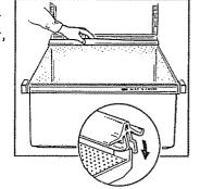
Then replace the light panel by hanging top of panel on upper pins and pushing in at bottom.
