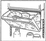
**To open,** push the latch up and pull the bin handle forward.
