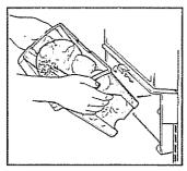
**To remove the bin,** lift it up and out of the bin housing.
