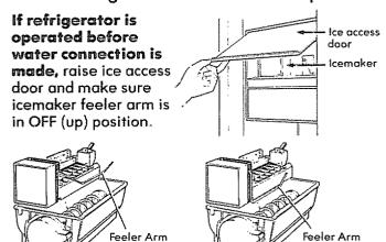
When water supply has been connected to icemaker, move feeler arm to ON (down) position.
