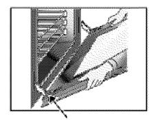
HINGE SLOT Door removed from the range
